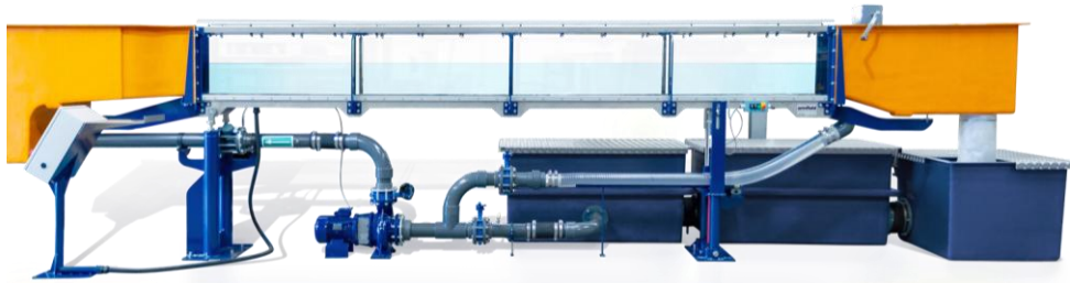
فلوم شیب پذیر 12*0.30*0.40 m Armfield S5/6- MKIII Standard teaching & research flume- tilting
